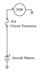
System wiring diagram for Dual SIM's (per engine)
