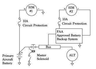
Each SIM consumes 1.5 amps of power and will deplete the main battery in the event of a generator or alternator failure even with battery/master switch OFF.
